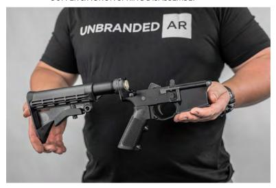
Warning: The buffer and action spring are under compression. Push down on the buffer retainer pin (A) while holding the buffer back. Allow buffer to travel forward slowly after clearing the retaining pin. Once the spring is no longer compressed, remove from buffer tube.
