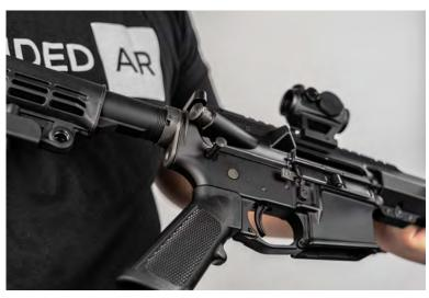
Grasp the rear of the upper receiver and pull up, allowing it to pivot on the front pin. This will expose the fire control group.
