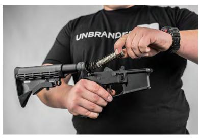
Clean inside of buffer tube with a cotton patch and CLP.
