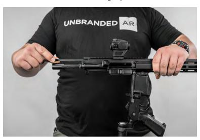
Pull the bolt carrier straight back until it is free of the charging handle and upper. Pull the charging handle back until it stops, then allow it to drop down to clear the upper receiver and remove it from the rear.
