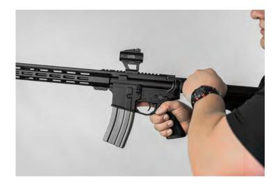
Unlock and pull the charging handle all the way out and press in on the lower portion of the bolt catch. Release charging handle. This locks the bolt in the open position.
